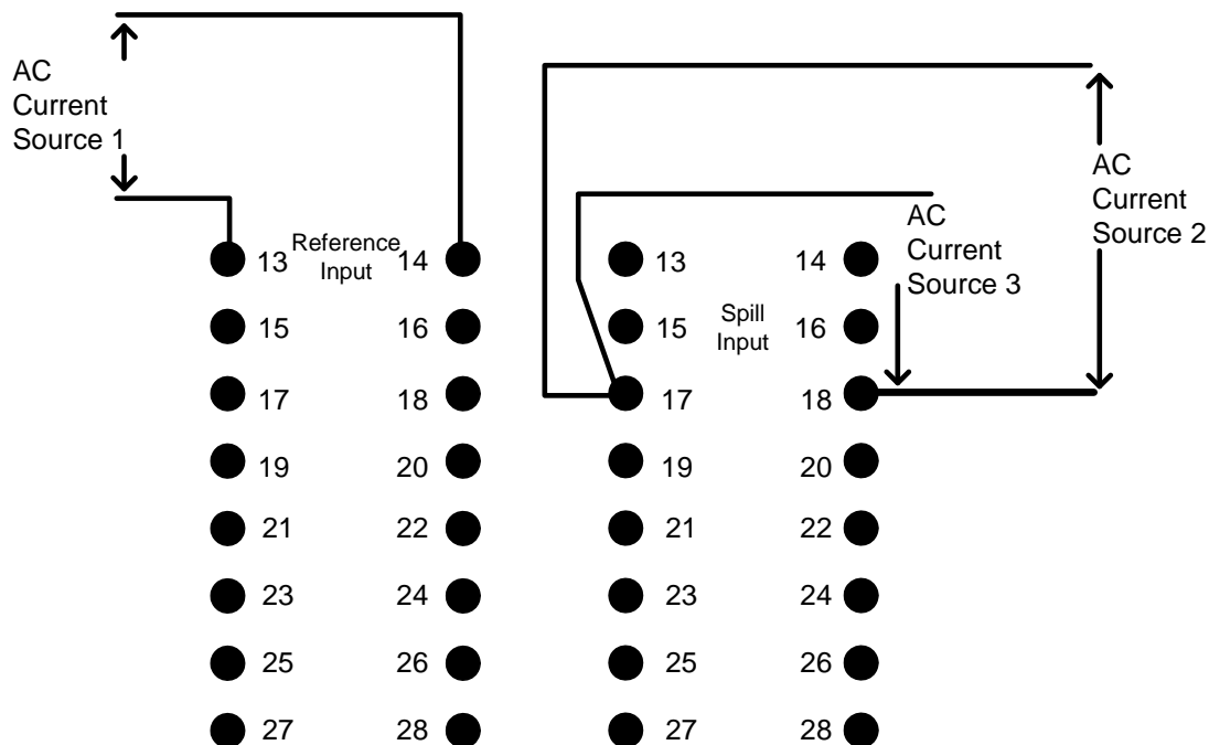
Figure 2 – C2 Unbalance Test Connection Diagram
